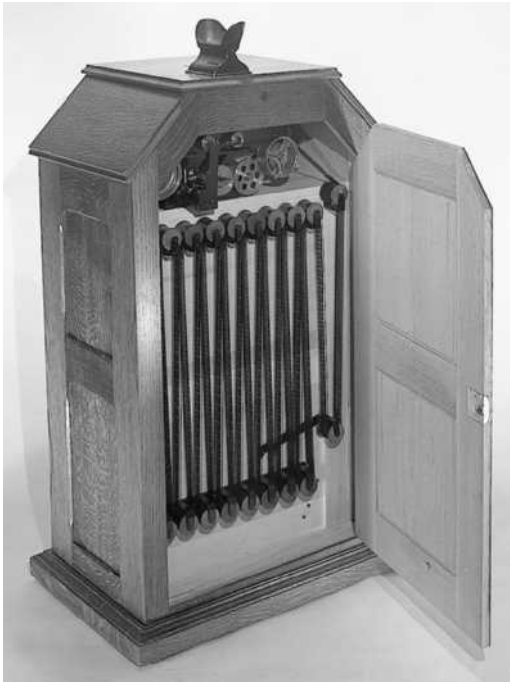
1.5 The Kinetoscope was a peephole device that ran the film around a series of rollers. Viewers activated it by putting a coin in a slot. (Source: George Eastman International Museum of Photography)
